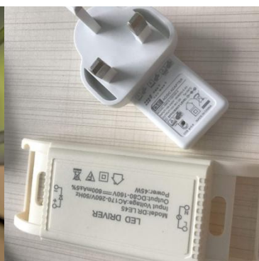
UV Laser marking on white pp plastic surface.
