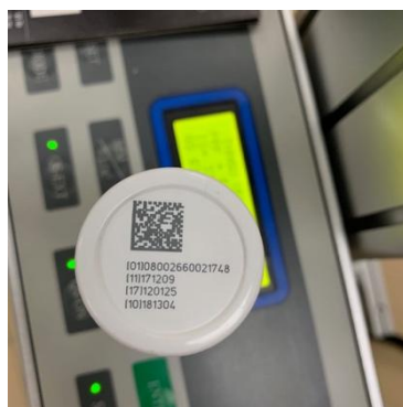
UV Laser marking on white pp plastic surface.
