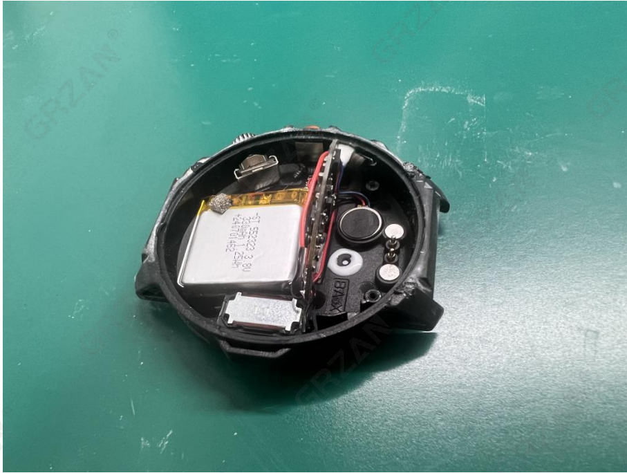
Photo 5: Visual inspection after the IP6X Test
