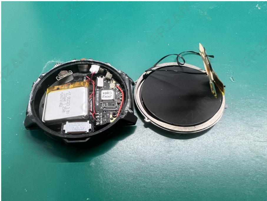
Photo 4: Visual inspection after the IP6X Test
