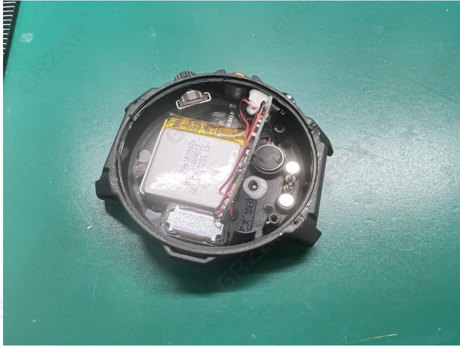
Photo 7: Visual inspection after the IPX8 Test
