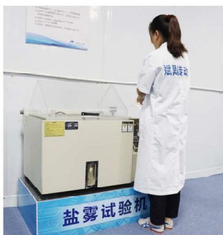
盐雾实验 Salt spray test
